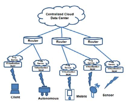
Figure 2. Proposed architecture for Cloud-Fog Computing
